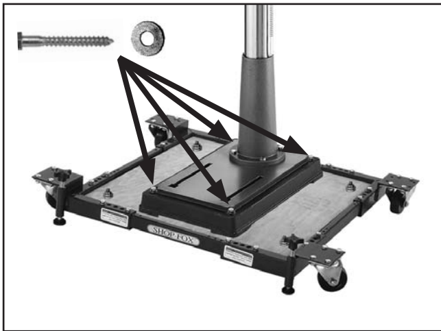
Figure 23. Drill press mounted on mobile base, using a base plate for support.
